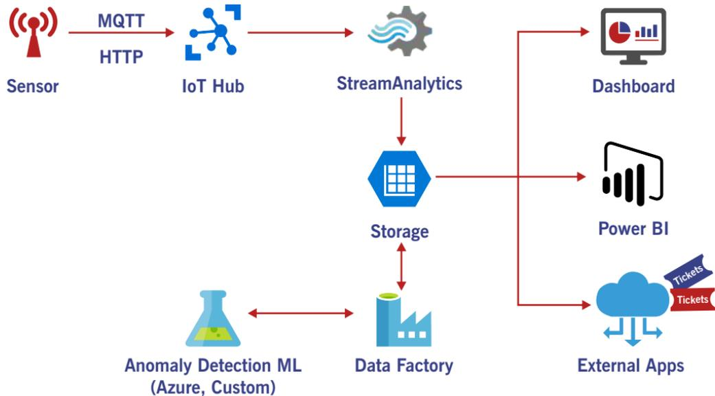
Figure 1. A typical Azure IoT Hub reference architecture of anomaly detection with Machine Learning
