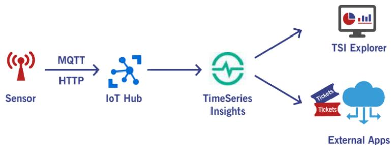
**Figure 3. A simple reference architecture of anomaly detection with Time Series Insights**
