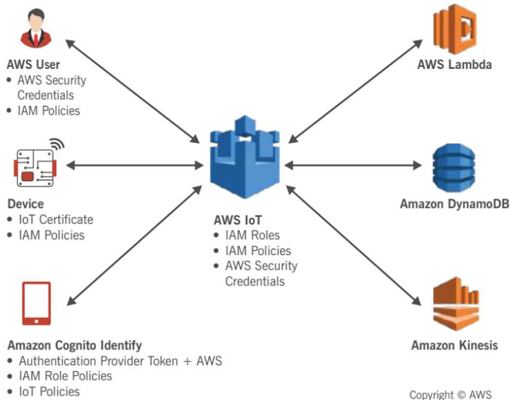
**Figure 2. IoT Security in AWS**
